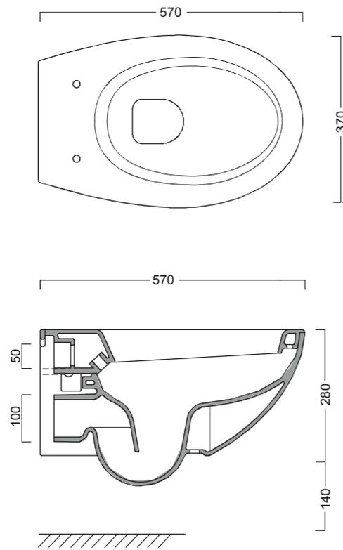
\* To be installed only on M12 bars |
